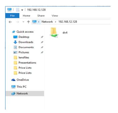
Copy the DV4home update file into the DV4 folder and reboot by disconnecting the power for 5 seconds.
