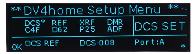
When you press and hold the MENU knob for selecting the reflector you will get back to the submenu. Turn the MENU knob for the next submenu selection, DCS Port and push the knob briefly. Select the desired port by turning the MENU knob and press and hold the MENU knob to complete the selection.
