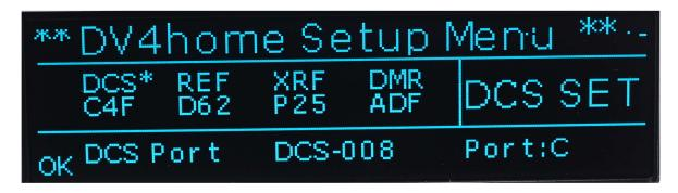
When you do a press and hold on the MENU knob for selecting the port it will bring you back to the submenu. Turn the MENU knob for the next submenu selection, Link DCS and push briefly. This completes the reflector selection and you are now connected.
