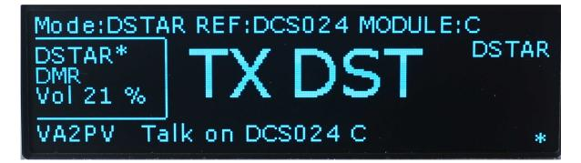
The last bottom line of the DV4home display gives you the current status on the reflector, showing the transmitting station, in that case it's VA2PV.
