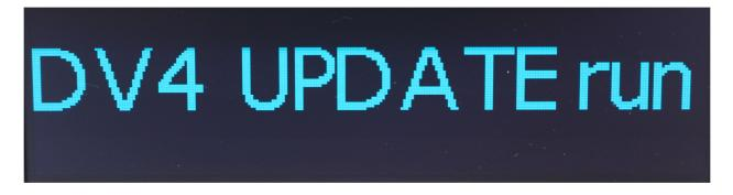
Every time you boot the DV4home it will show you the installed firmware version, so after upgrading make sure you have the new version active like below. If it's not the case, unplug the power for 10 seconds and reboot.
